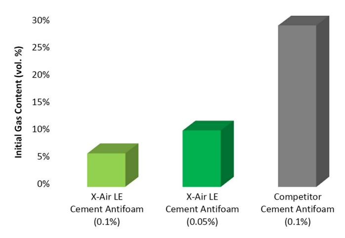
The X-Air LE liquid cement antifoam is more than five times as effective as the competitor at 0.1%. Even at half the concentration, X-Air LE cement antifoam is still over two and a half times as effective as the competitor.
