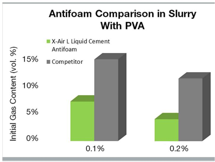
The X-Air L liquid Cement antifoam is over twice as effective as the competitor at 0.1% and almost four times as effective at 0.2%
