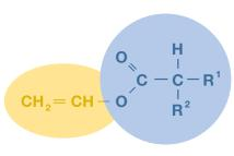
$R^1 = 4$  carbon atoms  $R^2 = 2$  carbon atoms
